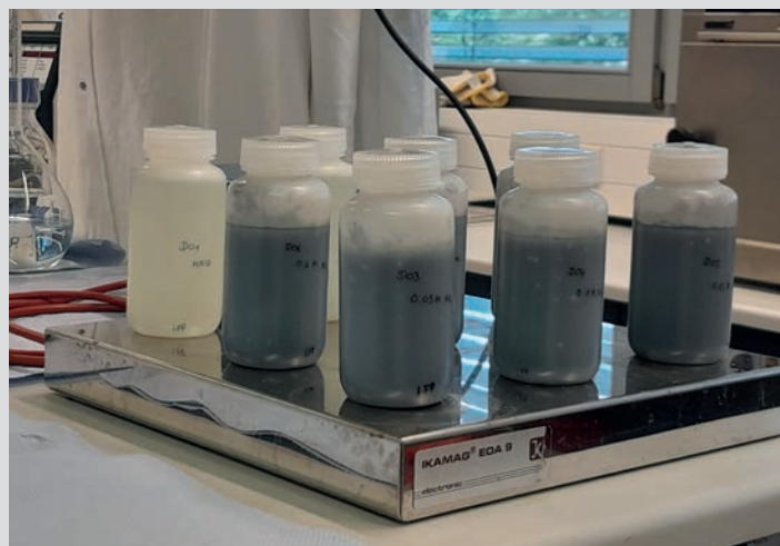
Samples in reaction vessels on a heated stir plate. Here, experiments with different weighted samples are made on the desorption of lithium from iron phosphate. The clear reaction vessels are so-called blanks, samples without iron phosphate, which serve to control the results. (Photo: R. Reich, KIT)
