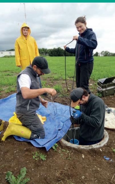
Installation of a seismometer in a borehole at the WINSENT test area near Stötten in the Swabian Jura. (Photo: KIT-GPI)
