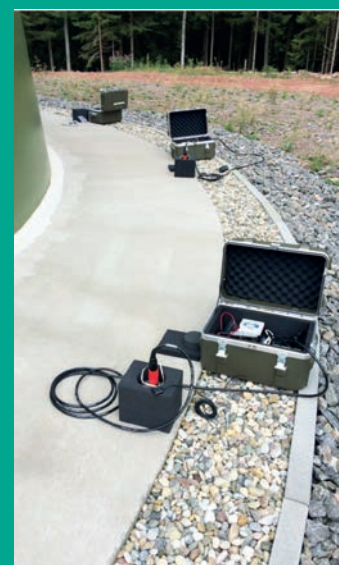
Measuring ground movements on the foundation of a wind turbine with a mobile seismological station. (Photo: KIT-GPI)
